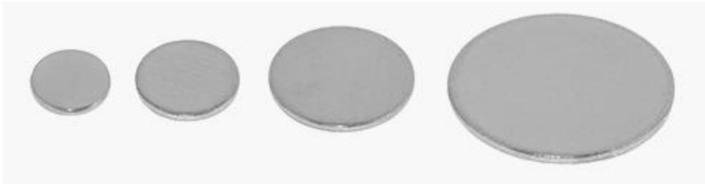
Magnetic metal specimen support discs are used on the AFM /SPM systems which employ a button magnet to hold the metal specimen disc. The metal specimen discs provided by NanoAndMore are made of a magnetic type 430 stainless steel with a nominal thickness of 0.90mm and a tolerance of +/- 0.08mm.
